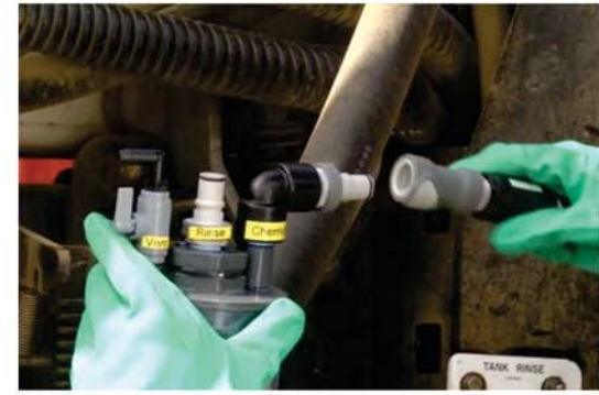
Connect chemical hose to pump and measuring device
