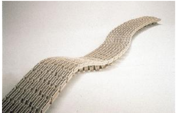
The sideflexing chain shown above features a unique ribbed surface for easy product transfers. It complies with FDA and USDA requirements for direct food contact. Celcon acetal copolymer was selected because of its low sliding friction and high strength.
