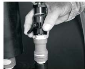
3. Open valve on rinse system; water pushes throughout the system
