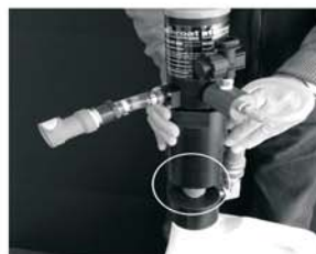
3. Disconnect pump from container assembly
